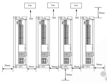
Figure 2.2: EM2RS series installation drawing
