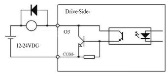
Figure 3.4: Output Interface Wiring
