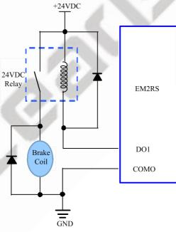
Figure 3.5: Brake output connection
